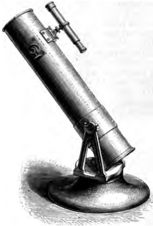
ALTAZIMUTH MOUNTING FOR A SMALL REFLECTOR.
